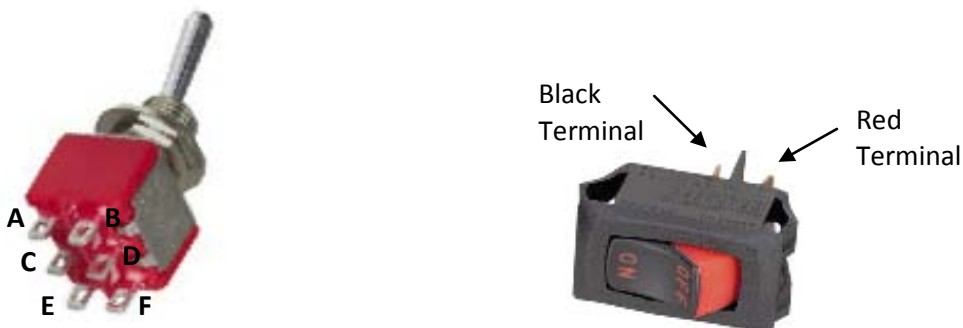
Figure 40. (LEFT) One of the DPDT switches, designated 'α', 'β' and 'γ' in Table 22. The letters A-F correspond to the nodes wires are to be soldered onto. (RIGHT) The Master Switch, designated 'δ' in Table 22.
