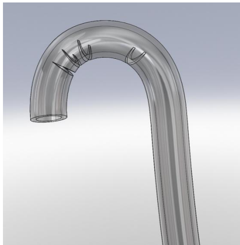
Figure 123: Wedge cuts to help bend Aorta
