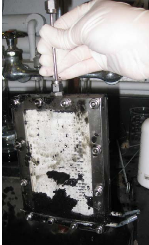
Figure 14: The membrane housing with the sparging tubes and bolt attachment
