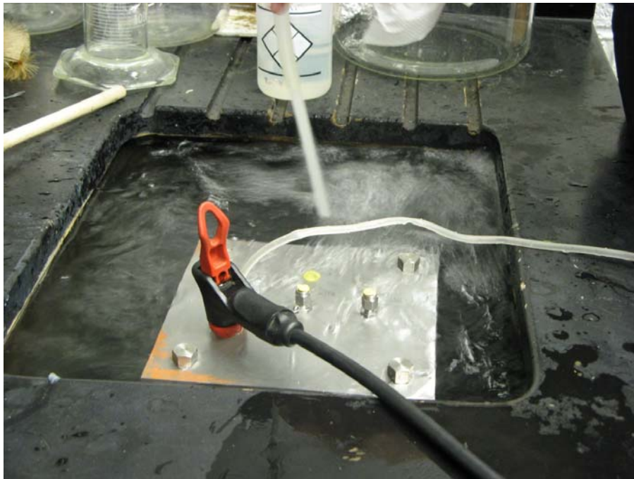
Figure 34: Air tightness testing was completed successfully while the vessel was submerged in water.
