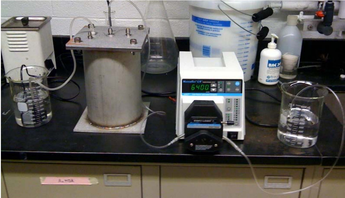
Figure 35: The setup for the flow validation and level sensor testing was completed successfully and is shown above. From left to right: source with example influent pump, MBAT vessel, example effluent peristaltic pump and drain.
