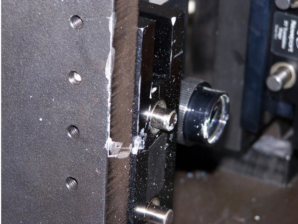
Figure O9: End of shaft deformed steel sensor mounts
