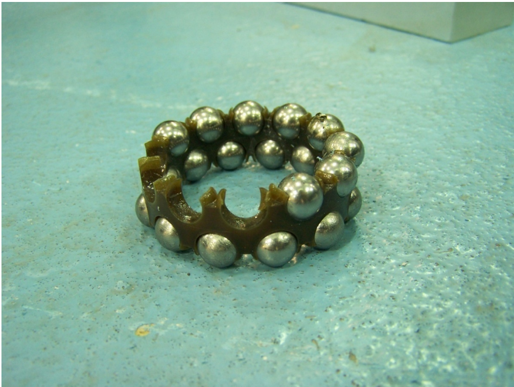
Figure O8: All but four of the ball bearings were recovered.
