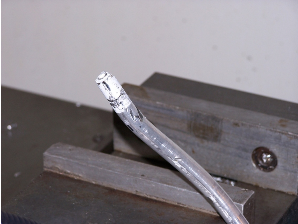
Figure O3: Deformed end of shaft
