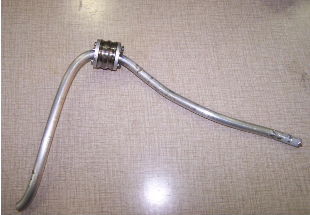
Figure O5: Deformed shaft with inner race of ball bearing, two bearing adaptors, and sleeve bearing
