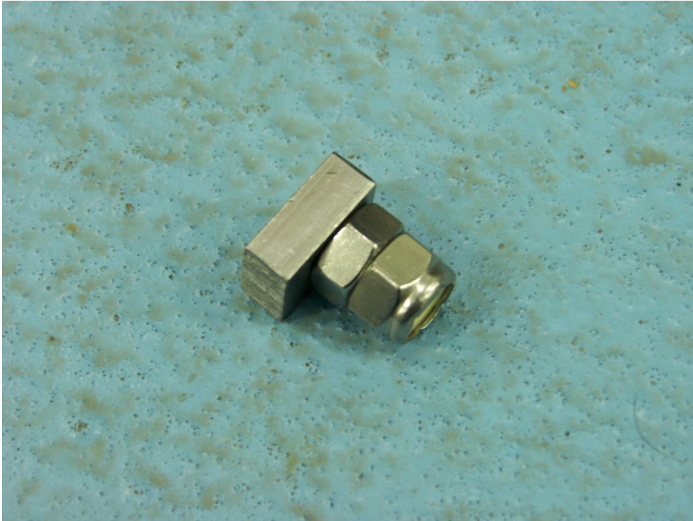
Figure O4: Threaded end of shaft with offset mass broke off the shaft
