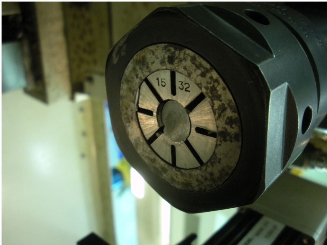
Figure O6: Fixed end of shaft remains in the mill collet.
