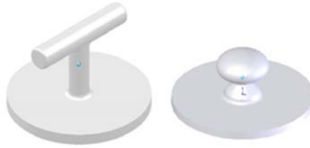
Figure 29: T-grip and knob alternate handle designs
