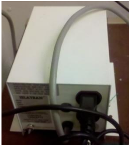
Islatran Isolation Transformer Model: LRAM-102 Input: 120 V Output: 120 V Freq: 60 Hz SN: 100078
