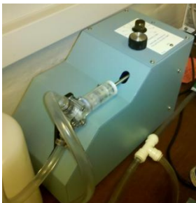
Harvard Apparatus Pulsatile Blood Pump Model: 1405-048 Max Current: 1 A (fuse) CAT # 55-1838 Input: 115 V, 50-60 Hz.
