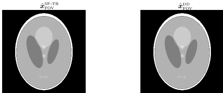
Figure 3.5: Axial views of FOV images \hat{x}_{\text{FOV}}^{\text{SF-TR}} and \hat{x}_{\text{FOV}}^{\text{DD}} reconstructed by the iterative method (PWLS-CG) using the SF and DD method respectively. Left : SF-TR projector; Right : DD projector.
