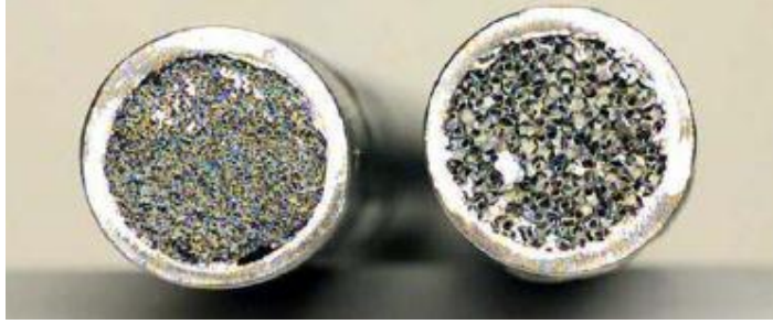
Figure 54: Open-cell metal foam pipes with different porosities [16]
