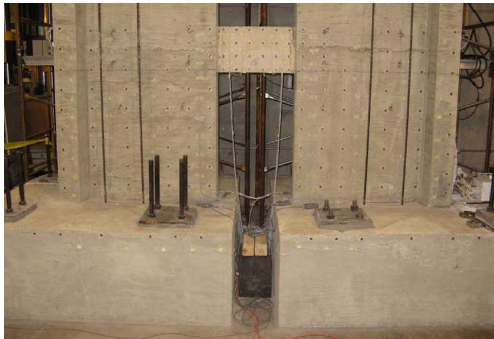
Figure 3.32 – Photo of optical system “marker” layout prior to testing
