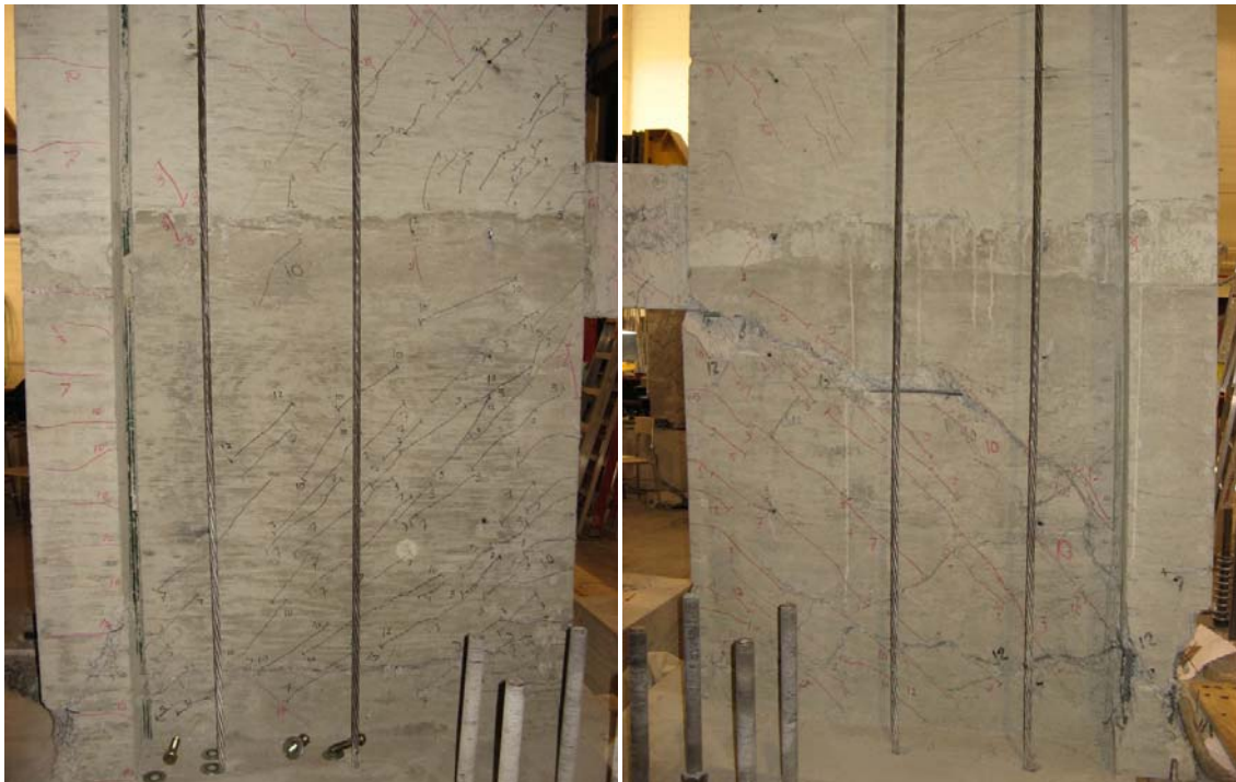
Figure 5.10 – Final damage state of the first story walls of Specimen CW-2 (left and right are east and west walls, respectively). Diagonal cracks occurred when each wall was in compression, flexural cracks predominantly occurred while wall was in tension.
