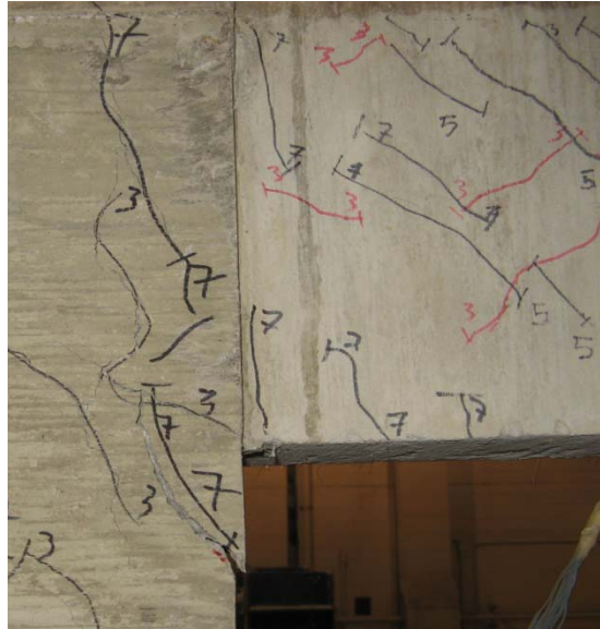
Figure 5.4 – Damage localizing along termination of longitudinal coupling beam reinforcement at 1% system drift (Specimen CW-1).
