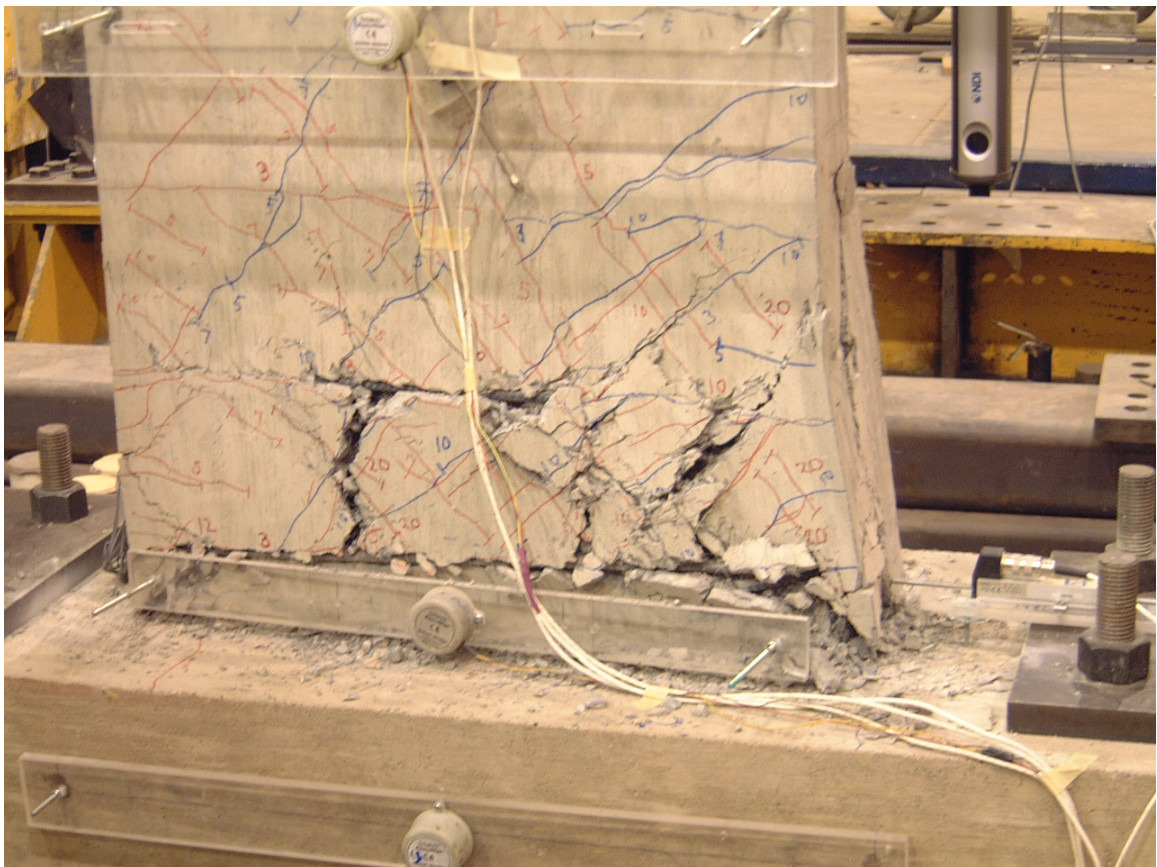
Figure 4.3 – Ultimate damage state of Specimen CB-1: insufficient confinement and sliding are evident
