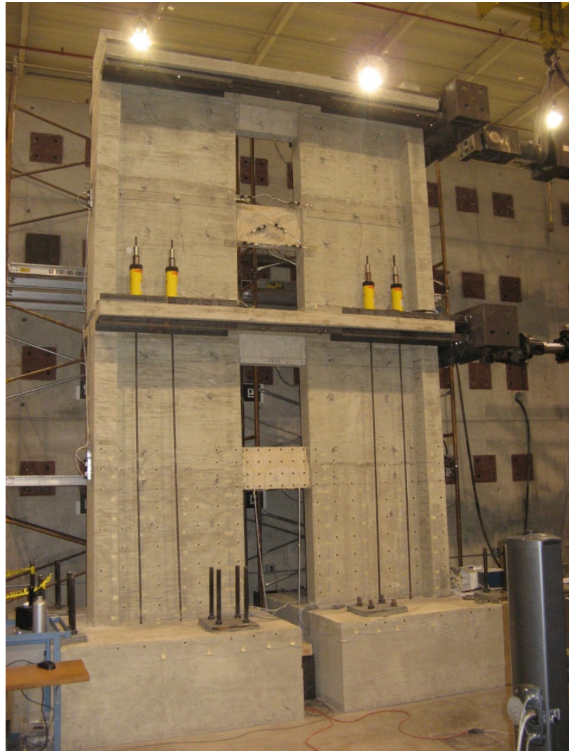
Figure 3.15 – Photo of coupled wall test setup and specimen
