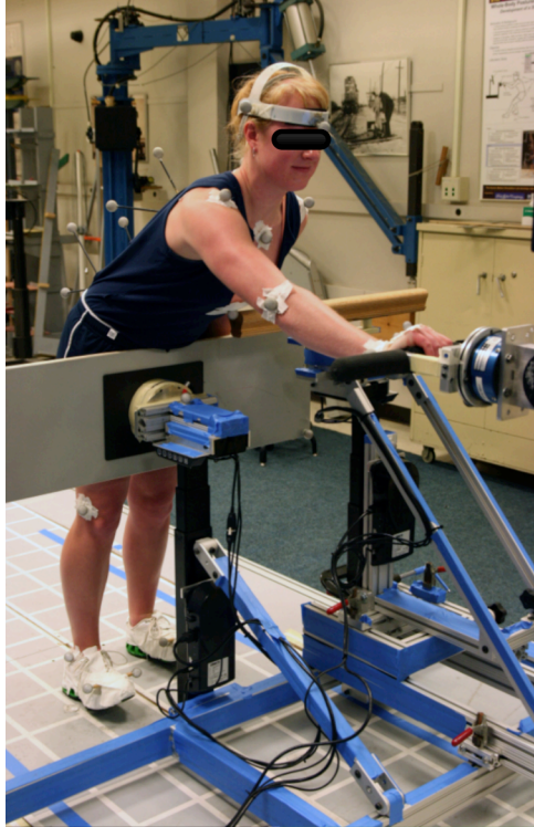
Figure 2.4.1. Subject performing an isometric exertion on the fixed task hand force handle while engaging the pelvis at the body-bracing support surface and receiving feedback on task hand force via an LCD screen.
