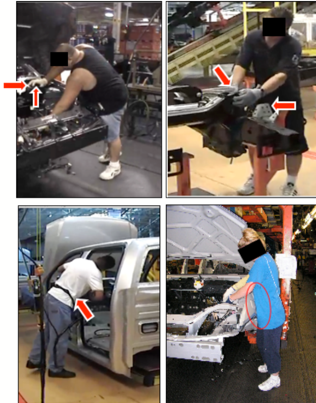
Figure 1.2.1 Representative automotive assembly tasks that involve kinematically constrained, approximately isometric exertions with bracing availability.
