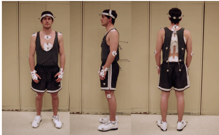
Figure 2.3.3. Retro-reflective marker set used to track whole-body postures and motion.
