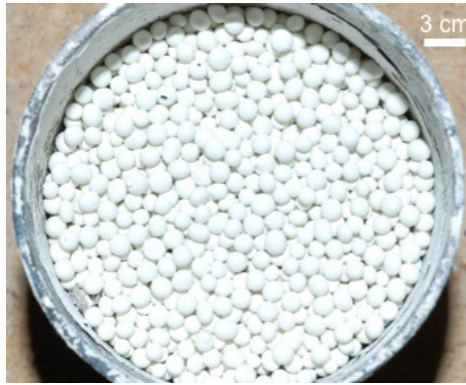
Figure 2.1 Ceramic beads comprised in the baffle used in the LMC casting process.
