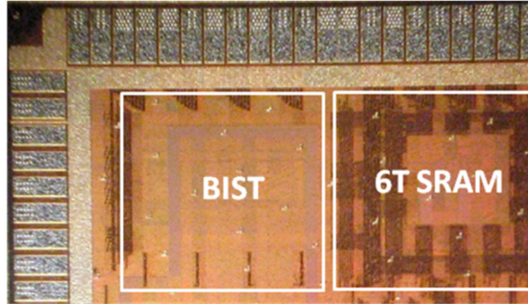
Figure 8.2 Die-shot of the 45nm test chip showing the SRAM array and built-in self-test (BIST) structure.
