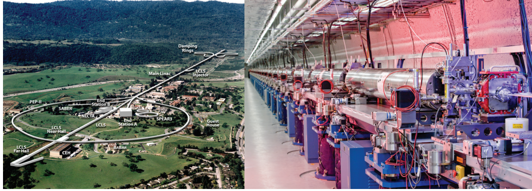
Figure 1.1: The Linac Coherent Light Source upgrade replaced the final kilometer of SLAC with an undulator and additional experimental facilities. The 132 m long LCLS undulator at SLAC. Images courtesy of the SLAC National Accelerator Laboratory.
