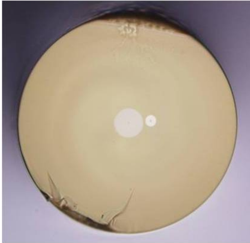
Figure 1.1: Cross-section view of CCC fiber sample with 250\mu\text{m} -diameter cladding, 35\mu\text{m} -diameter central core, 13\mu\text{m} -diameter side core, 0.06 central core NA, and 0.1 side core NA. The separation between central core and side core is 3\mu\text{m} , and the helix pitch of the side core is 6.1mm.
