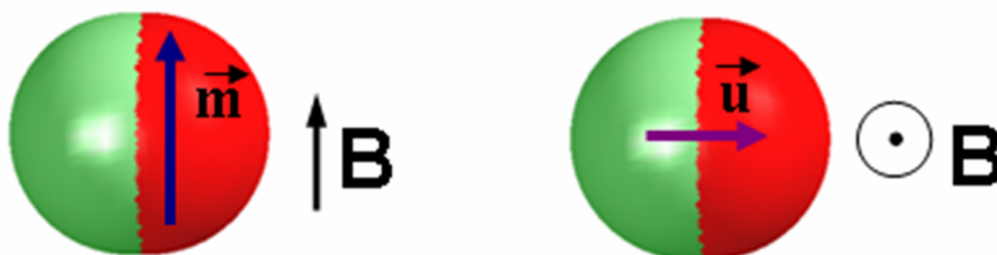
Figure 6.18 Model magnetic Janus particle. The red hemisphere represents the magnetic compartment containing magnetite nanoparticles. Left: Side view. The blue arrow indicates the induced magnetic dipole \mathbf{m} not coincident with the particle center and aligning with the field vector. Right: Top view. The orientation vector \mathbf{u} is in the x-y plane and perpendicular to the field vector.
