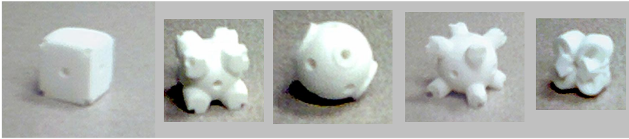
Fig. 6. Photos of selected quasi-Pareto optimal shapes that were rapidly manufactured using selective laser sintering
