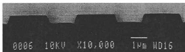
Figure 1. Cross-sectional view of 4 \mu\text{m} period Si relief grating. We estimate the structure as: period=3.96 \mu\text{m} , top linewidth = 2.2 \mu\text{m} , depth = 0.52 \mu\text{m} , and wall angle = 73.9°.
