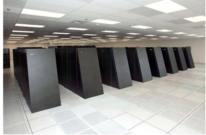
IBM’s Blue Gene P supercomputer, capable of a sustained speed of 1 petaflop—roughly the speed of the human brain
