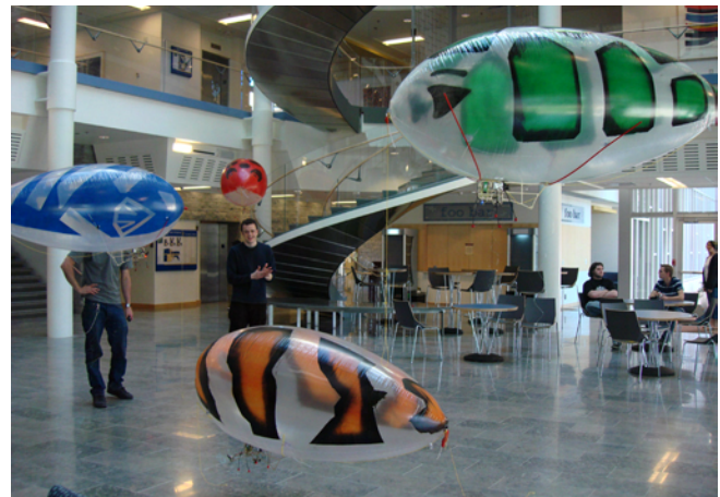
Another example of active student learning: a fleet of autonomous dirigibles that exhibit flocking behavior...
