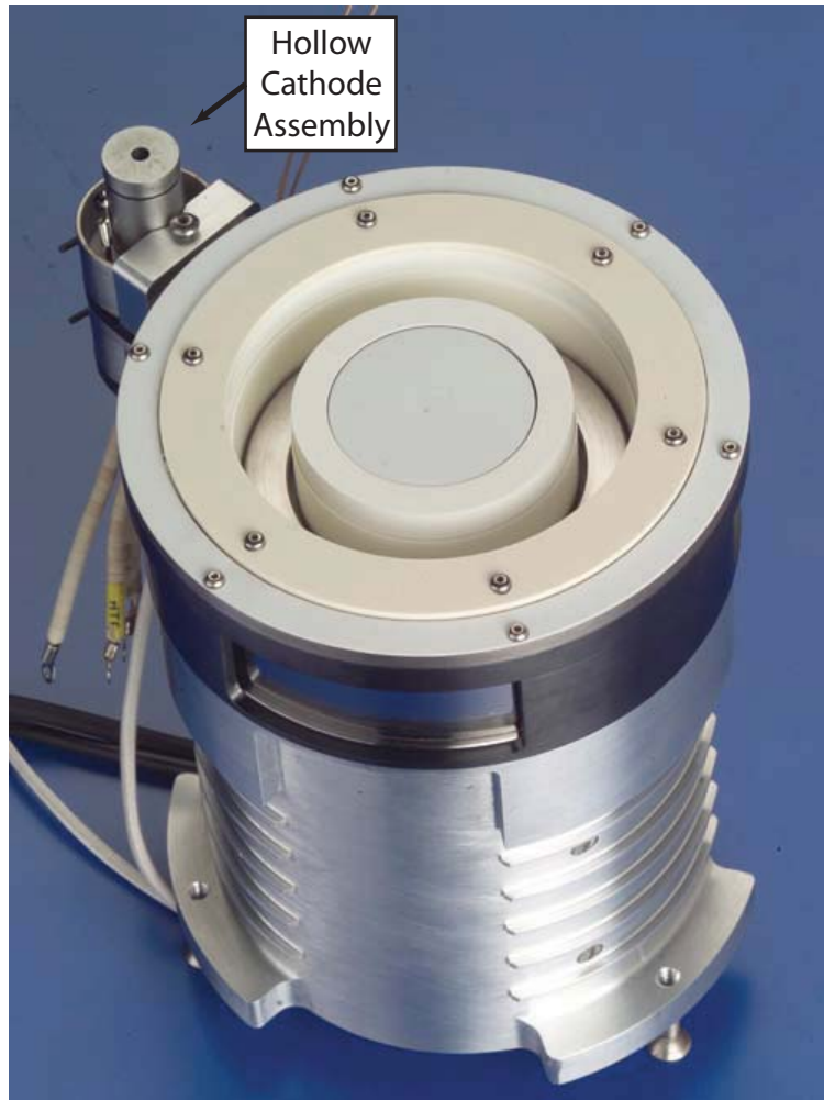
Figure 2.3: Photograph of HCA mounted with the NASA-103M.XL (HiVHAC) prototype thruster. Image from [38].
