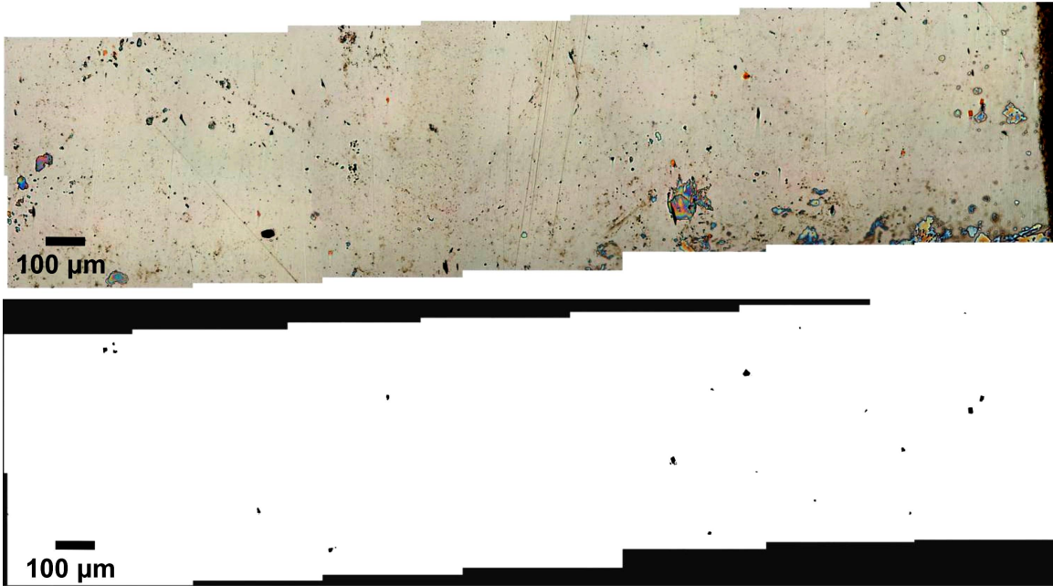
Figure 5.10: (Top Image) Photostitched collection of optical micrograph of polished 4330 steel collected from a random 2D cross-section in the bar-end of a double-linear shear test specimen. Cuboidal titanium nitrides were segmented out from thunder-represente matrix using basic thresholding algorithms and gaussian filters to create a binary image (Bottom Image).
