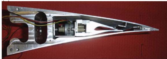
Figure 1.7: A linear actuator system for microflaps implemented at the UC Davis Aeronautical Wind Tunnel Facility [27].
