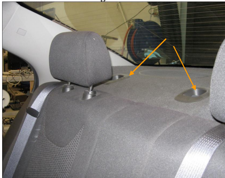
Figure 3. Tether anchorage locations and headrests in upright position for CRS installation as directed by vehicle owner's manual.
