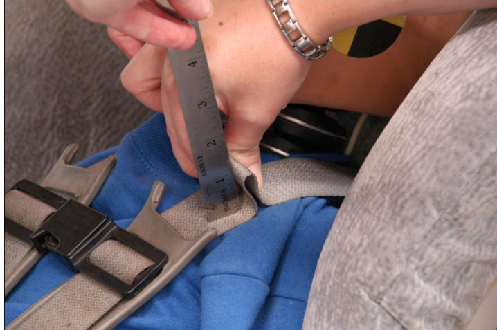
Figure 8. Measuring amount of harness slack.
