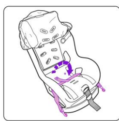
Figure 56. Illustration of combined labels dealing with belt routing from ComfortSport.
