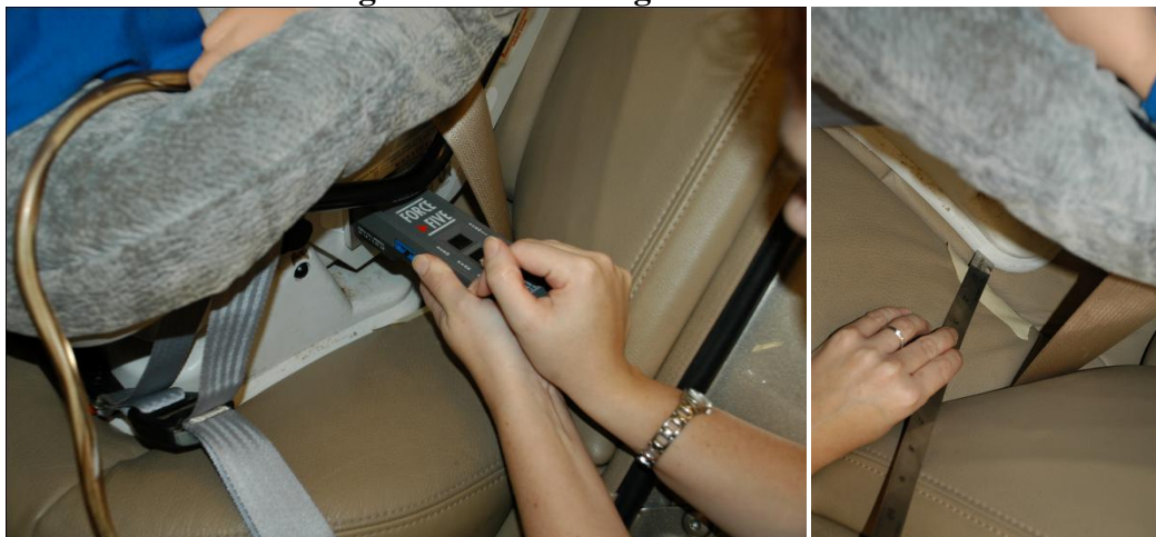
Figure 10. Measuring amount of CRS lateral displacement under applied load.
