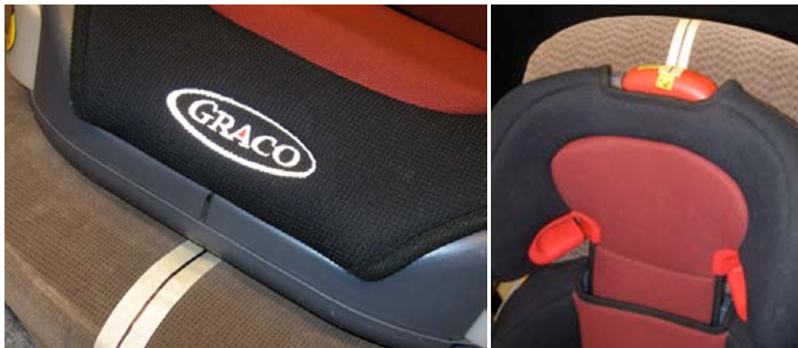
Figure 19. Aligning center planes of booster and vehicle seat
