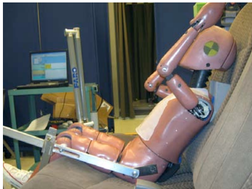
Figure 33. Propping ATD head off the seat back
