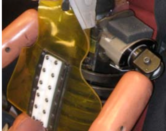
Figure 16. Example of ½ inch thick shoulder spacer
