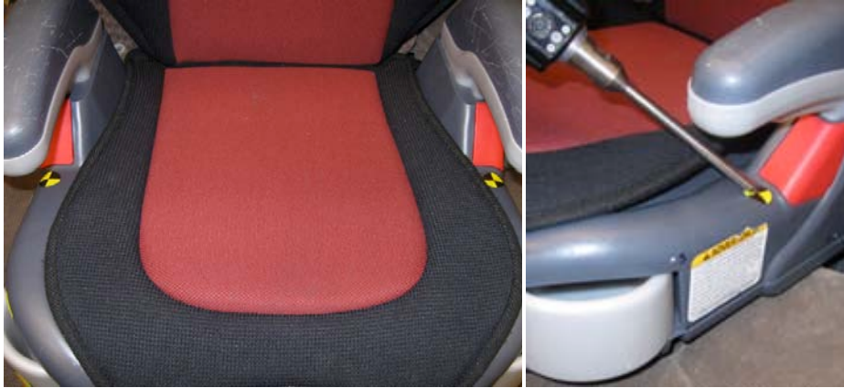
Figure 17. Example bilaterally symmetrical points on booster seat
