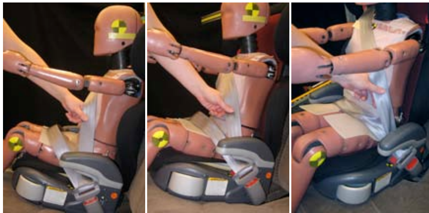
Figure 40. Point at which the lap belt is released (left) while pulling on the shoulder belt in the direction of the belt path until slack is removed from lap belt.
