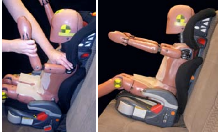
Figure 34. Keeping clavicles down and back while rotating arm downward.
