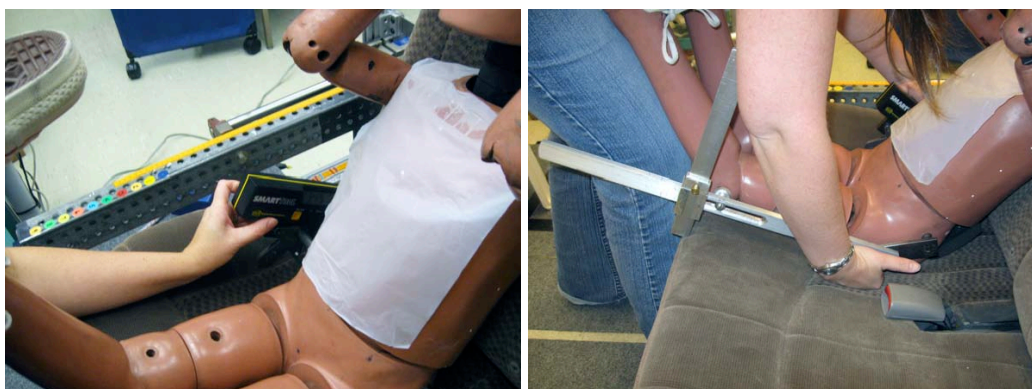
Figure 31. Moving the pelvis forward
