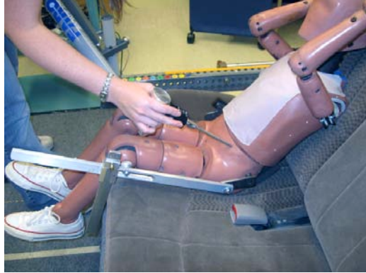
Figure 32. Checking ATD pelvis position
