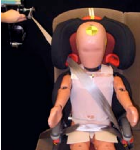
Figure 41. Feeding the shoulder belt into the retractor
