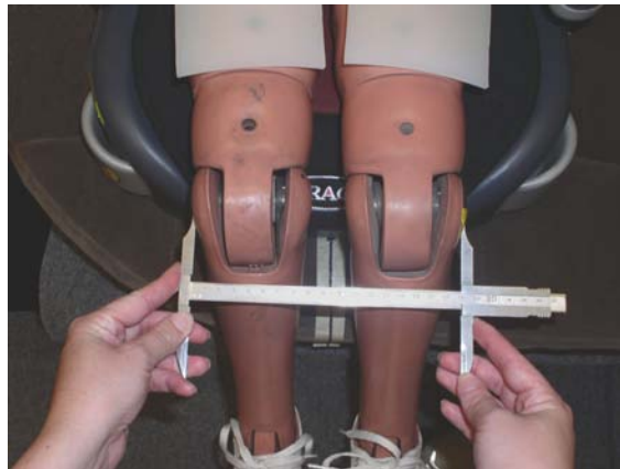
Figure 35. Setting the distance between the outer edges of the knees to 180 mm for the six-year-old and 220 mm for the ten-year-old.
