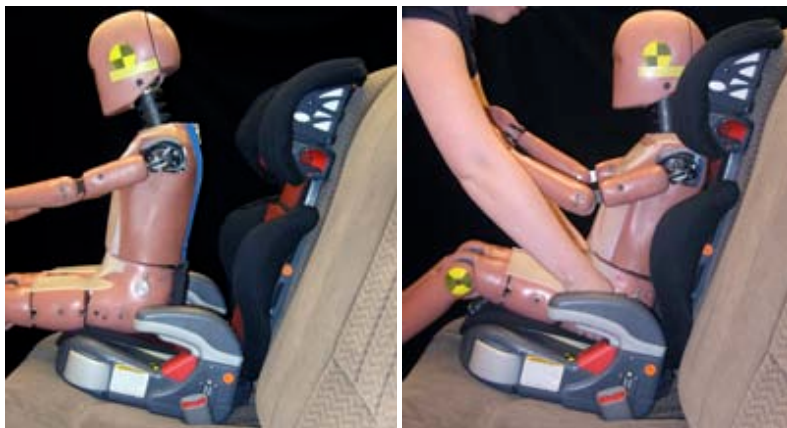
Figure 22. Moving the ATD rearward in the seat
