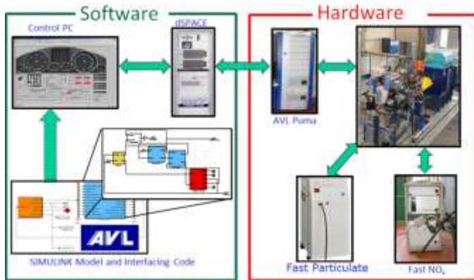
Figure 2: Engine-In-the-Loop test cell configuration
