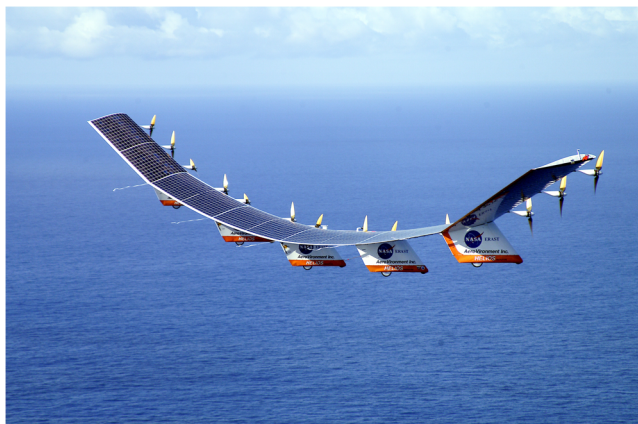
NASA Dryden Flight Research Center Photo Collection http://www.dfrc.nasa.gov/gallery/photo/index.html NASA Photo: EDO1-0209-2 Date: July 14, 2001 Photo by: Nick Galante/PMRF The Helios Prototype flying wing is shown over the Pacific Ocean during its first test flight on solar power from the U.S. Navy's Pacific Missile Range Facility in Hawaii.
