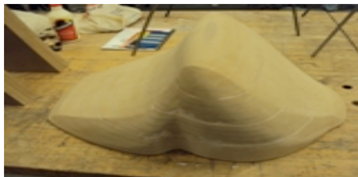
Illustration 2: The mold was designed in the Rhino Cad, and the file transferred to the CNC Router where the mold was constructed.
