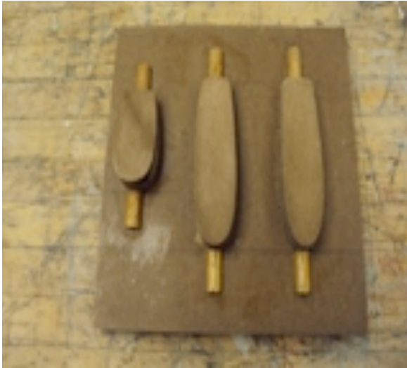
Illustration 6: The Shock Mount file was transferred to the CNC Router where the mold was created. The wood mold was then used to create a plastic mold using the vacuum forming procedure. The dyed rubber was poured into the plastic mold creating the shock mounts.
