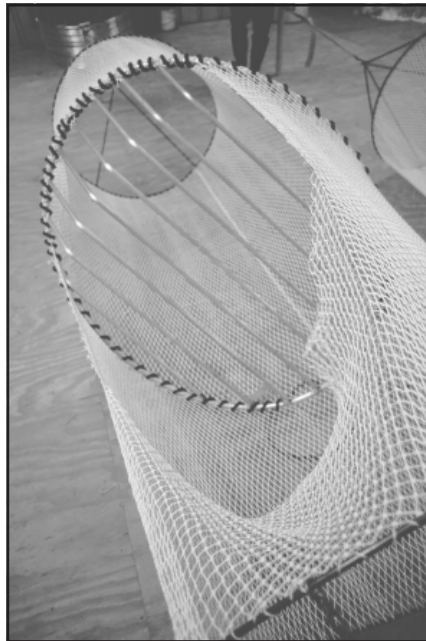
Figure 1. Turtle excluder device (TED) manufactured by Saunders Marine Machine Shop. The oval metal ring and bars deflect the turtles. The cut in the netting is where the trap door will be placed. The bars force a turtle to the trap door which will open allowing the turtle to go free. Photo by Bob Williams, NOAA.
