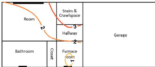
Figure 5-4. Floor plan of House 1 showing the spatial distribution of TCE vapor concentrations: (a) sampling locations and corresponding TCE concentrations (ppb) determined by Proto 1 and by canister/TO-15 (in parentheses); and (b) kriged contour map of TCE concentrations (ppb) in the basement showing the gradient with distance from the primary VI entry location in the crawlspace.
