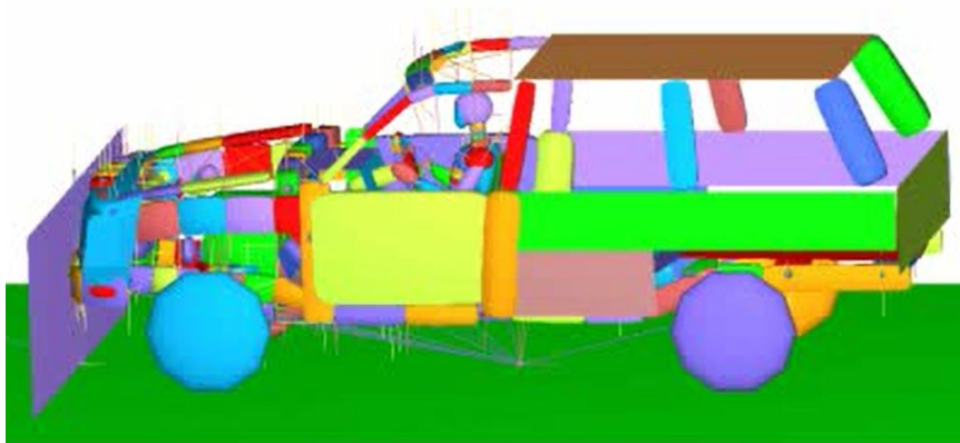
Figure 3.2: MADYMO-based vehicle simulation model of a 1995 Ford Explorer with mid-size male occupant
