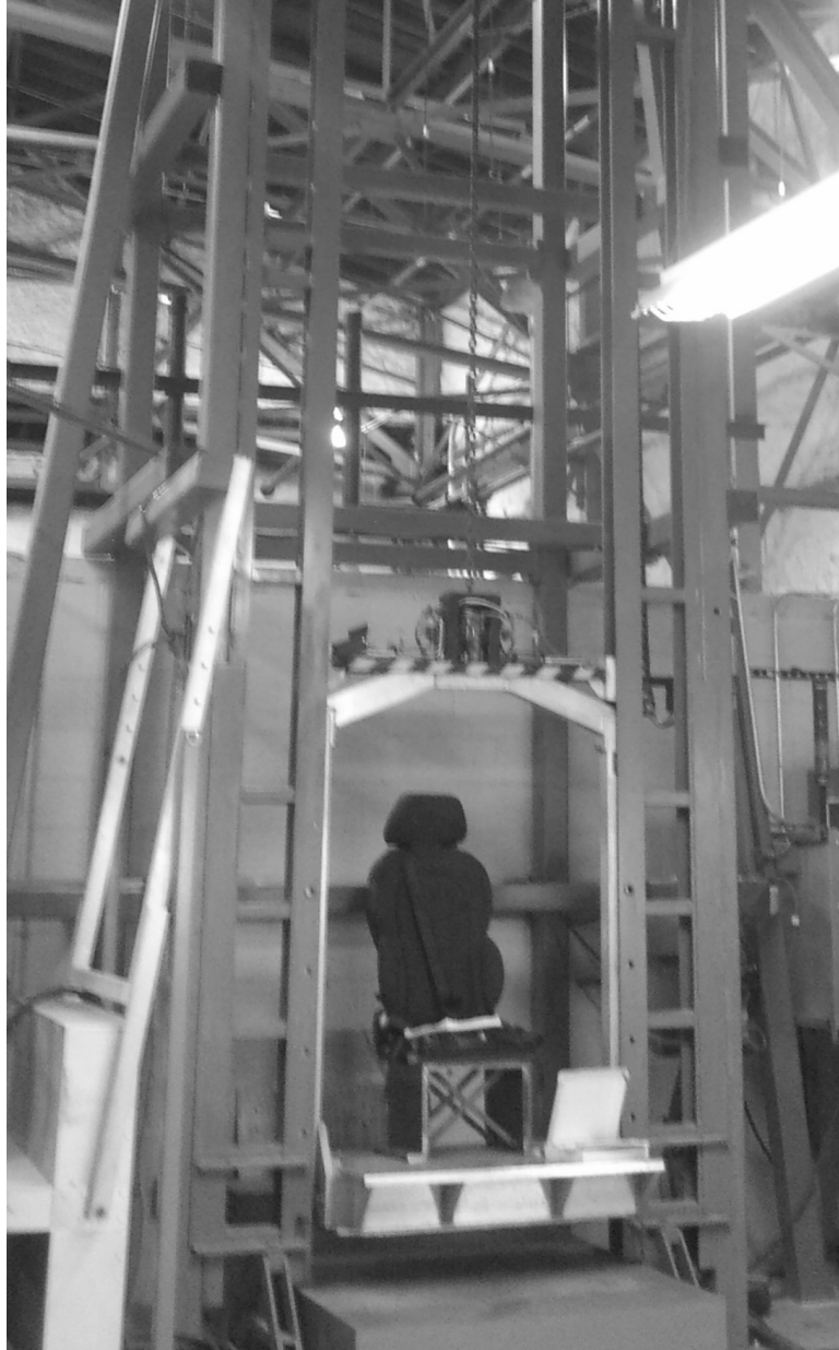
Figure 4.2: Photograph of the physical drop tower set-up at the Selfridge Air National Guard Base
