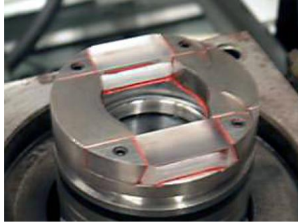
Figure 22: Picture of the bowl shaped piston. Optical access is achieved through an axial window and two side windows which allow access into the bowl.
