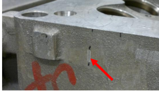
Figure 54: A light sheet of approximately 140 \mu\text{m} FWHM thickness, 6 mm width, at 10 mJ had sufficient energy density to ablate material off of a spare cylinder head.
