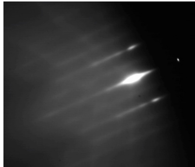
Figure 1.4: RHEED pattern of a GaAs buffer surface showing x2 periodicity.
