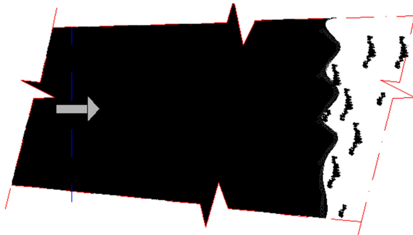
Figure 2.28 – Stage IV, maximum cavity length. The cavity now extends almost the full length of the beach flat. The cavity edge shape fluctuates rapidly. There is erratic shedding of wide, but short, clouds. (Figure by Mr. Andrew Wiggins. Reproduced with permission.)
