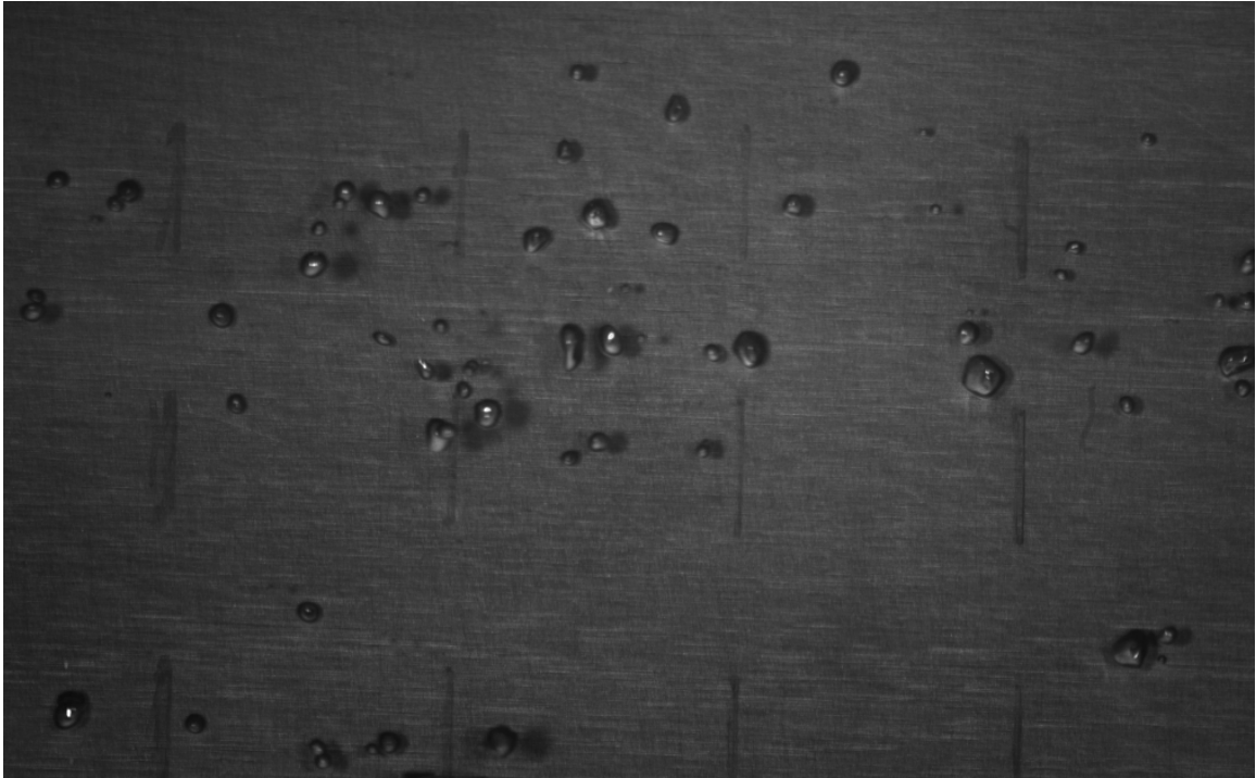
Figure 6.23 – Still photograph from a 1000 fps movie showing the bubbles near probe position #2 as viewed from below. The dashed lines are spaced on average 2.54 cm apart.
