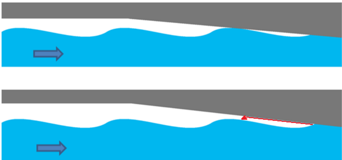
Figure 2.4 – Conceptual sketch of potential cavity closure events leading to shedding of gas. The upper illustration depicts the pinching mechanism, the lower the re-entrant jet process, where the red arrow moving upstream represents the re-entrant jet.
