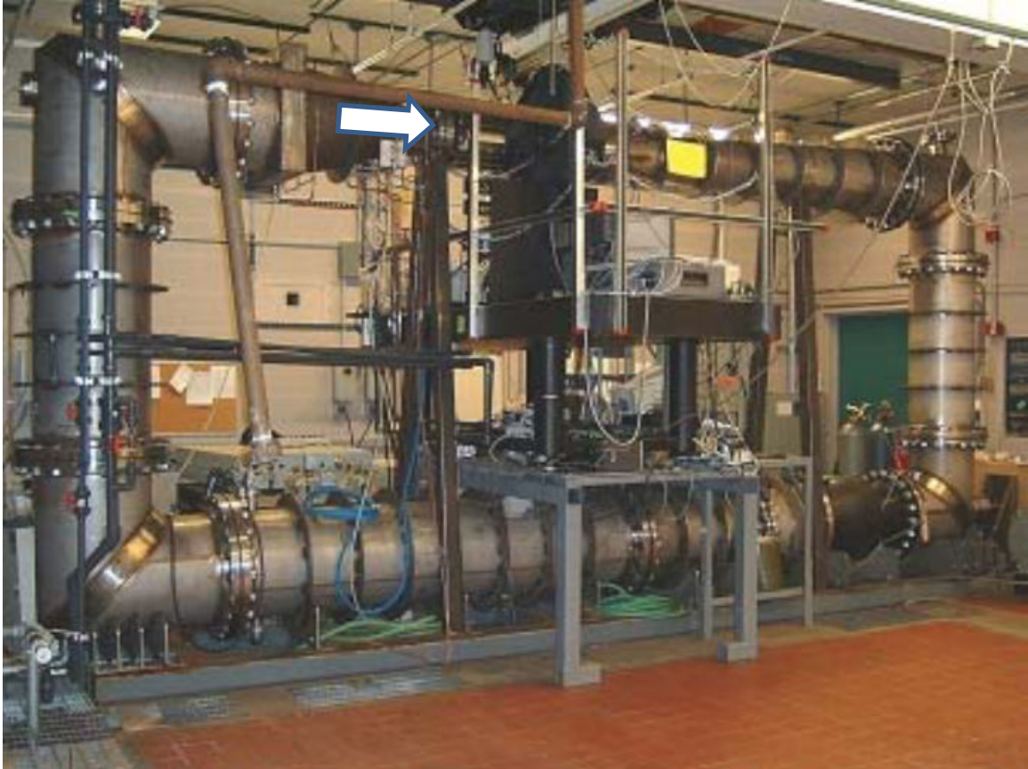
Figure 5.5 – The University of Michigan’s 9” water tunnel before construction of the new platform. A 12 ft x 18 ft test stand capable of accommodating the lead shielding’s weight and size was designed by the author. The white arrow shows the direction of the flow and also points to the test section.
