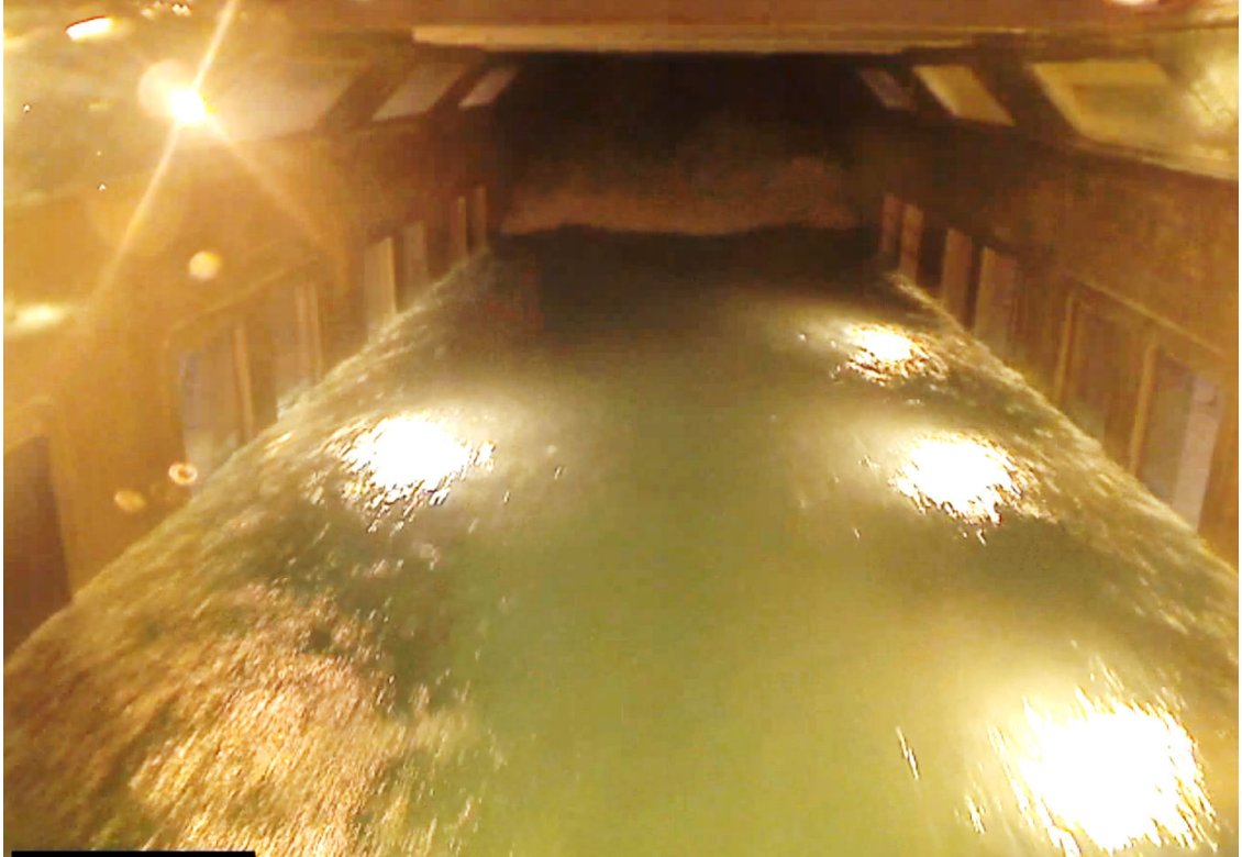
Figure A.19 – Looking downstream the free surface can be seen to have become flat and free of major perturbations, providing a suitable surface for free surface testing. The hydraulic jump which terminated the free surface in this case was just after the test section and can partially be seen.
