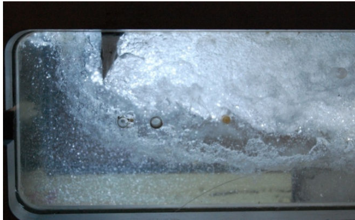
Figure A.6 – The old version of the gate in the MLCC and a loss of cavity.
