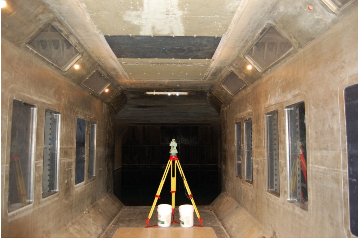
Figure A.7 – Looking upstream inside the LCC's test section. Leica measurement station seen in the middle of the image.
