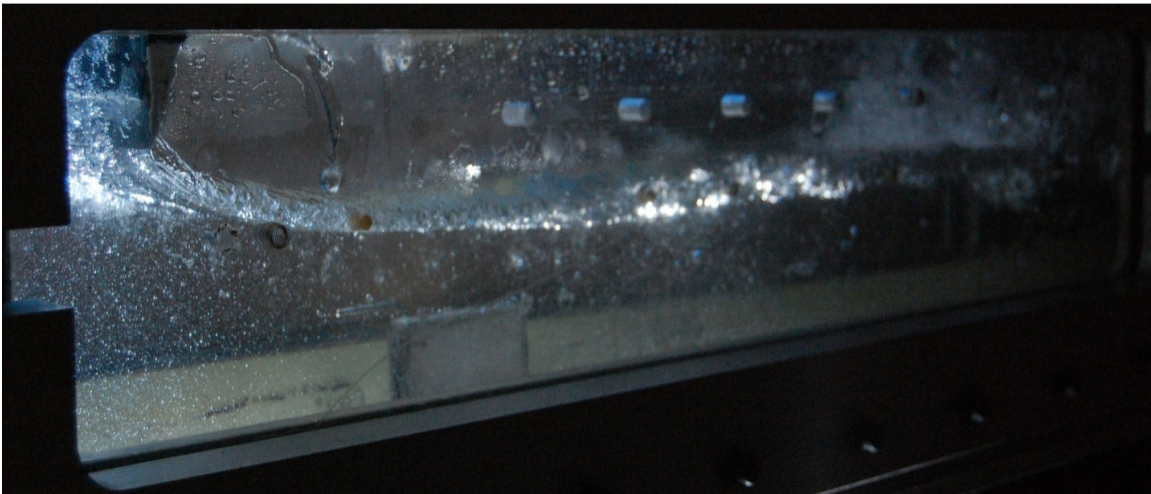
Figure A.2 – Oblique view of the gate and free surface. U = 2.5 m/s, Fr = 2.7 ( Fr -scaled for LCC: 9.4 m/s), old version of the gate in fully vertical position. The pitot used to measure the flow speed and its foil shaped support can be seen in the middle of the image. The frothy region near the aft of the test section is due to water draining down from hoses that connected the volume in front of the gate to the end of the test section, allowing air accumulating in front of the gate to be removed.
