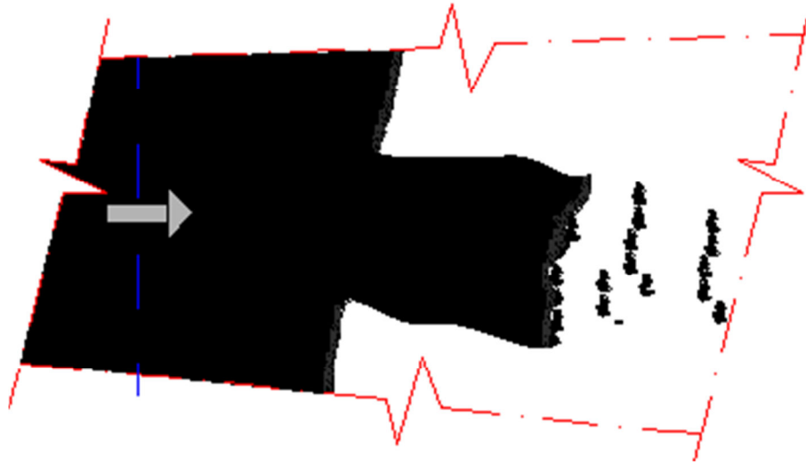
Figure 2.29 – Stage V, beginning of the retreat. Necking of the fully extended closure region initiates near the sidewall resulting in substantial variations in closure position. (Figure by Mr. Andrew Wiggins. Reproduced with permission.)
