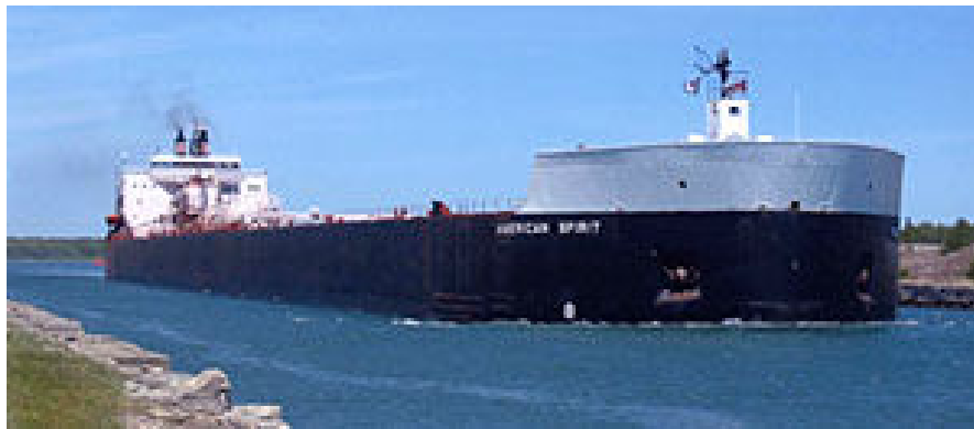
Figure 4.3 – The M/V American spirit is a cargo ship operating on the U.S. Great Lakes. L= 306 m, w= 32 m and midsummer draft 8.8 m (American Steamship Company).
