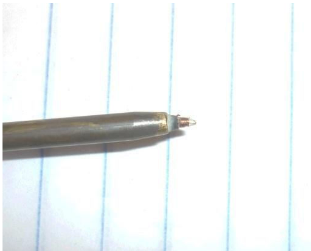
Figure C.3 – A close up of the point electrode. The thicker support is 1/8" in diameter, the excitation was provided by the electrode at the very tip and the sensing was done via the middle conducting copper color ring seen between the black and white insulating material.
