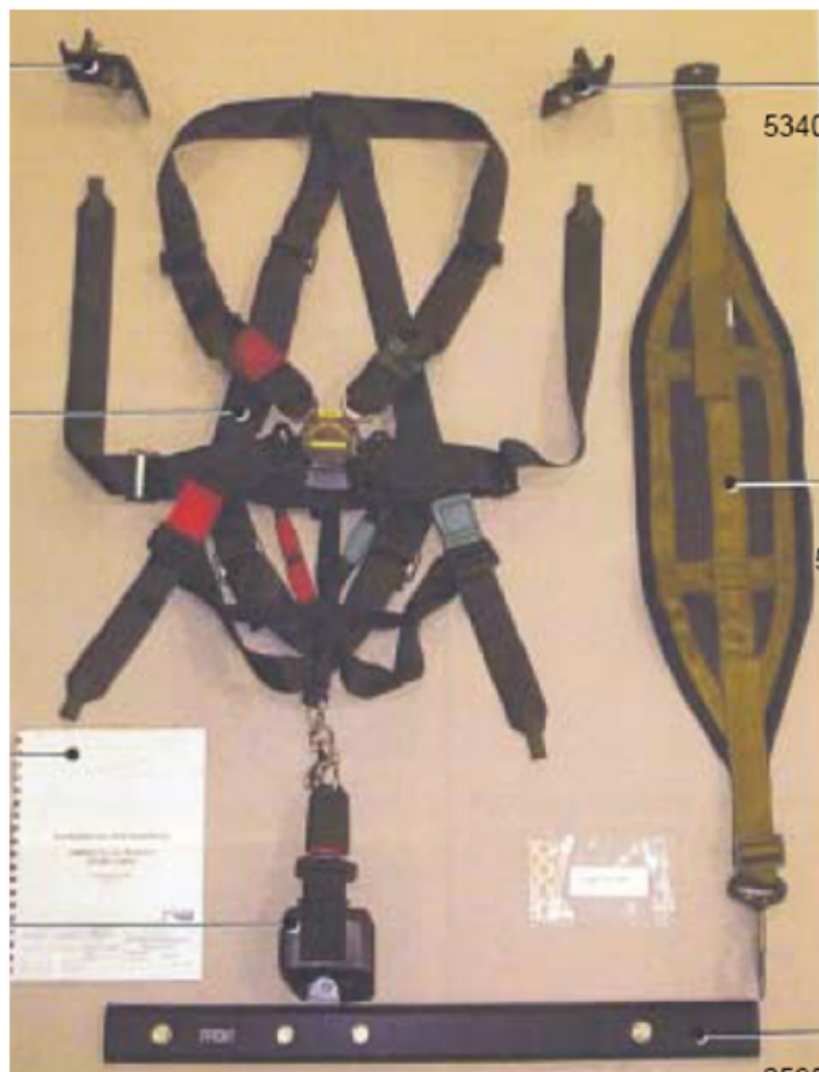
Figure 1.12: Components of the improved GRS ( Olive Drab website )
