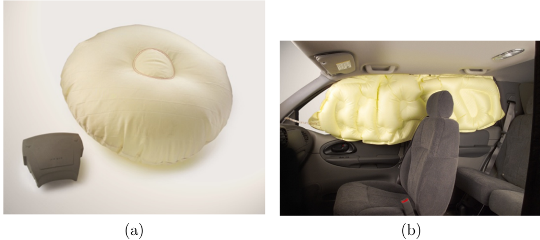
Figure 1.7: (a) Driver side airbag module (b) Deployed curtain airbag (Delphi website)
