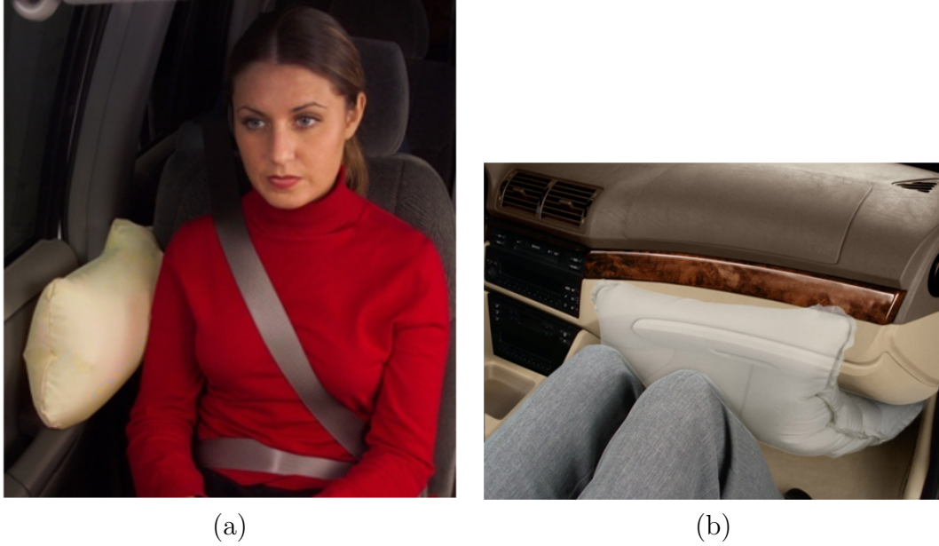
Figure 1.8: (a) Deployed torso airbag (b) Deployed knee airbag (Delphi website)
