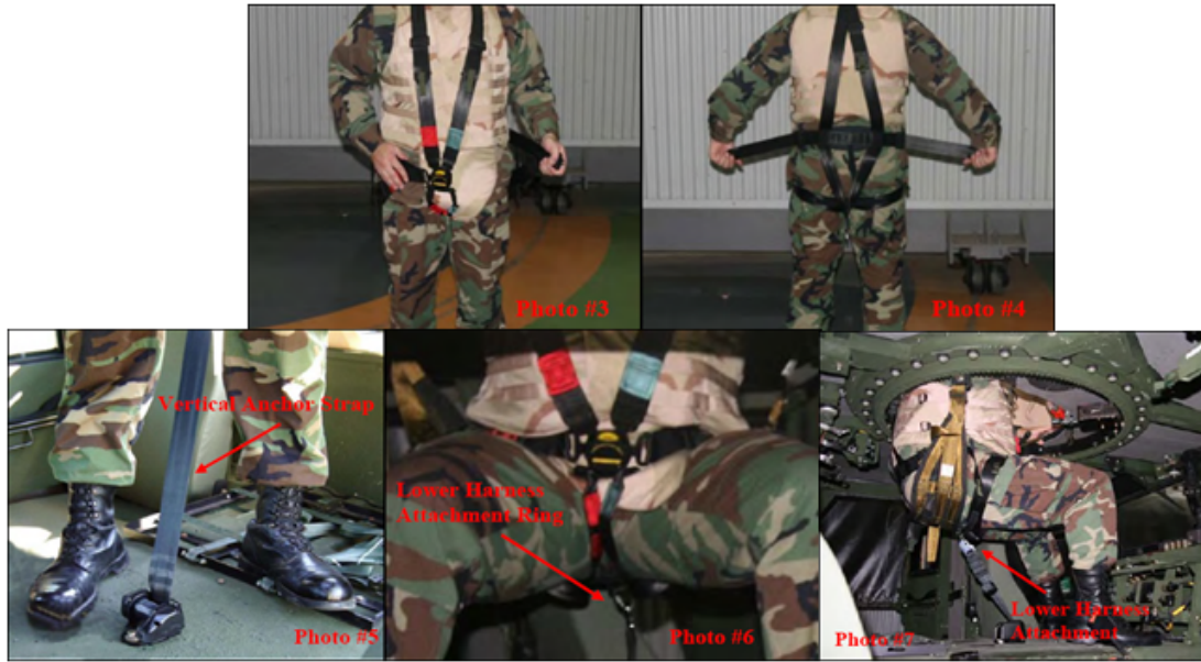
Figure 1.10: Single anchor GRS developed by Schroth ( Carr, 2006 )
