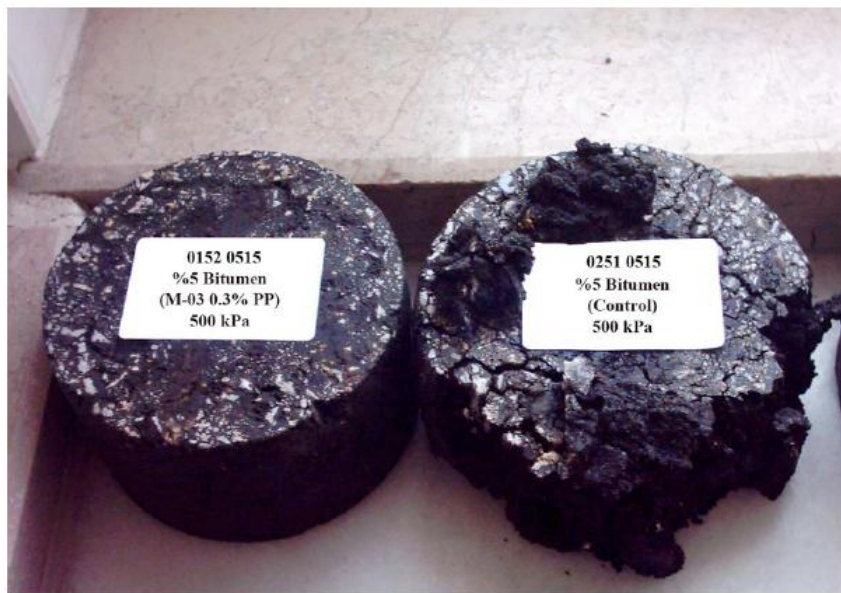
Fig. 2.2 Picture representing final conditions of control and polypropylene fiber reinforced specimens (Tapkin et al. 2009)
