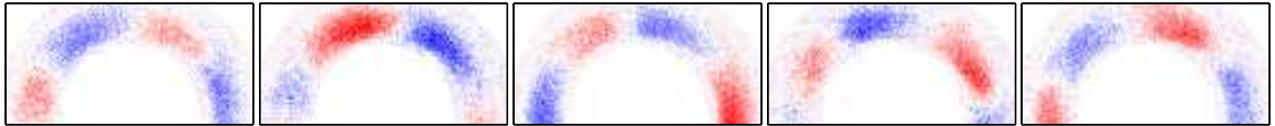
(b) NASA 173Mv1 (partial image) with a m = 3 mode at 300 V, 7 A, 45000 fps
