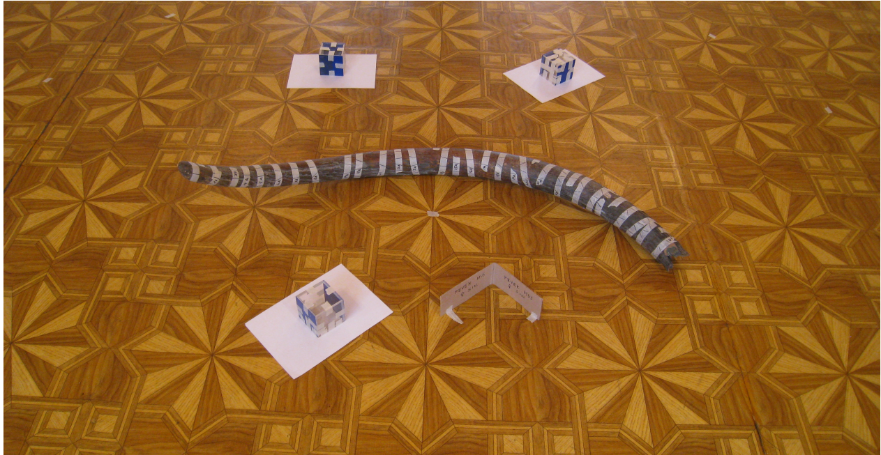
Figure 1 – Pevk 1, the most extensively prepared tusk, as seen in an image used to generate its model. This is taken from the highest camera height and includes all the points used as references. The cubes are 8 cm on a side and each had the top four corners used as references and to scale the project. The centers of the geometric starbursts were also used as references. Photo and tusk preparation by Dan Fisher.
