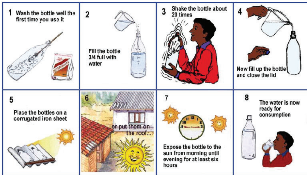
Figure 61: Disinfection using a clear, unscratched plastic or glass bottle (Meierhofer, 2006)
