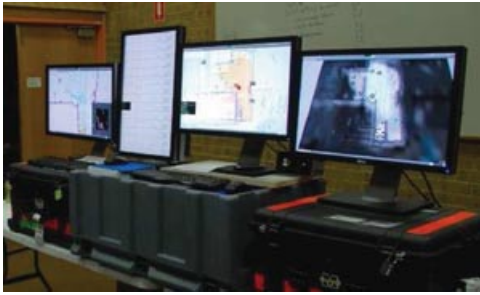
Figure 17. Team Michigan's user interfaces (from left): SOC, Status Dashboard, TOC, and SAGE. These are shown in greater detail in Figures 19 and 20.
