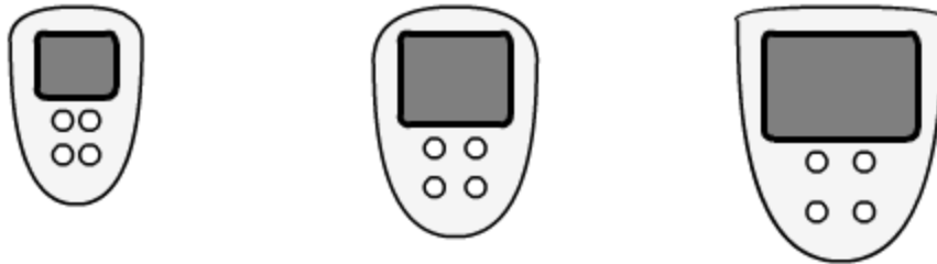
Figure 4.6. Select glucose meter designs, from left to right; the smallest final generation design selected, the mean design across all participants, and the largest design across all participants.
