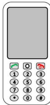
Figure 2.1. Mobile phone design using mean measured values reported in Table 2.3. This phone is sized to have the mean proportions of all of the phones measured in the literature.
