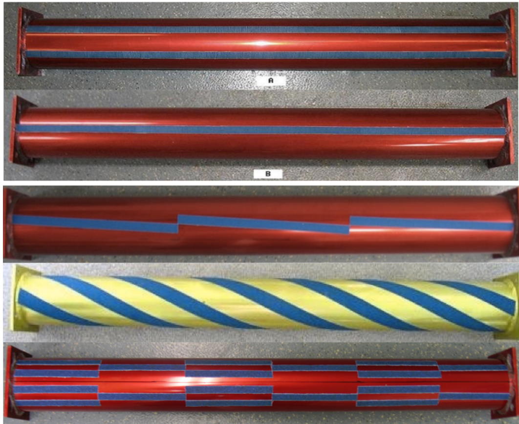
Fig. 2.4. Pictures of PTC configurations. From top to bottom: two straight roughness strips, one straight roughness strip, T7, T6 (helically applied strip), T8 (staggered strip)
