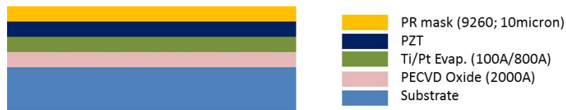
Fig. A.4 Layers of test samples for PZT etching experiment
