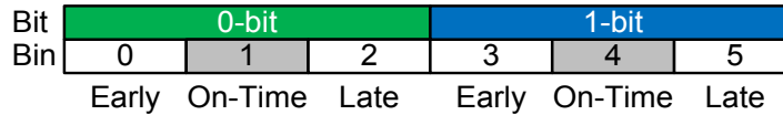
Fig. 5.3. Pulse-position modulation divides time into two timeslots for 0-bit and 1-bit. Those timeslots are sub-divided into three bins (early, on-time, and late) for clock tracking by the receiver.
