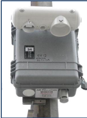
Figure 7. Portable Air Sampler Used by the NYC Community Air Survey to Measure Street Level Air Quality at 10-12 Feet From the Ground.
