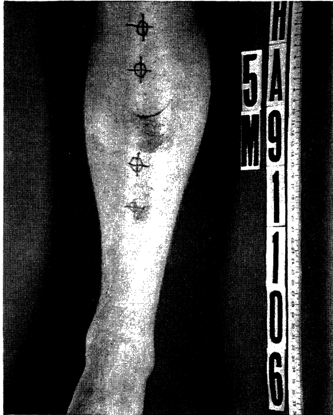
Figure 13. Post-test photo of ARS 3 injury produced by 40-L airbag at 200 mm.
