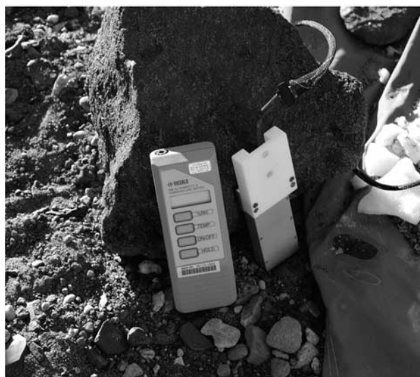
Figure 14. (left) The TECP deployed in Beacon Valley. (right) Needle 3 temperature and bulk dielectric permittivity recorded during the overnight hours of 2 January 2008.
