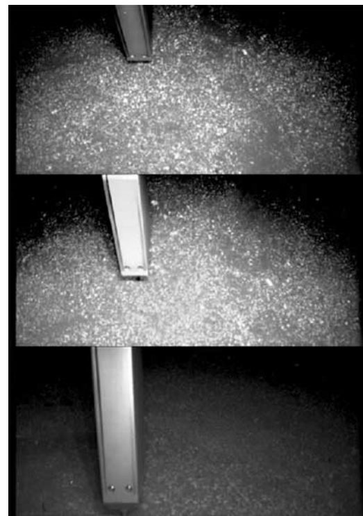
Figure 16. The RAC view of the TECP at insertion angles of (top) 30^\circ , (middle) 47^\circ , and (bottom) 77^\circ .
