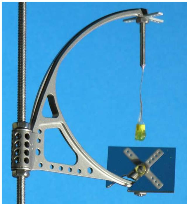
**Figure 1.** The Telltale assembly. The total height of the instrument is 83.1 mm. Lightweight Kapton tube (yellow) is suspended in braided Kevlar fibers ( $\sim 40$  fibers of  $18 \mu\text{m}$  in diameter). The Kapton part is viewed both directly and by mirror image from the below. Note that in this image the (flight unit) Telltale is mounted on a threaded pin and not on top of the meteorology mast.
