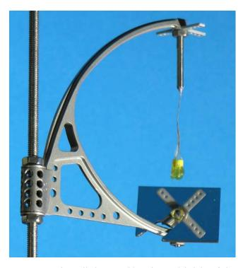
**Figure 1.** The Telltale assembly. The total height of the instrument is 83.1 mm. Lightweight Kapton tube (yellow) is suspended in braided Kevlar fibers (~40 fibers of 18  $\mu$ m in diameter). The Kapton part is viewed both directly and by mirror image from the below. Note that in this image the (flight unit) Telltale is mounted on a threaded pin and not on top of the meteorology mast.
