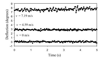
Figure 4. Typical time series from wind tunnel experiments obtained at the wind speeds indicated. These data were taken at orientation  $\beta = 39.2^{\circ}$  and P = 14 mbar air.
