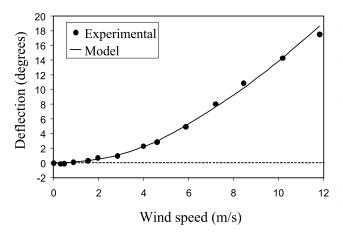
**Figure 5.** Representative deflection as a function of wind velocity. Data were obtained at orientation  $\beta = 39.2^{\circ}$  and P = 14 mbar air. The solid line shows model prediction as described in the text.
