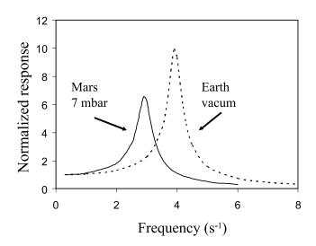
**Figure 7.** Calculated frequency response of the Telltale deflection under vacuum conditions on Earth and in 7 mbar pressure on Mars.
