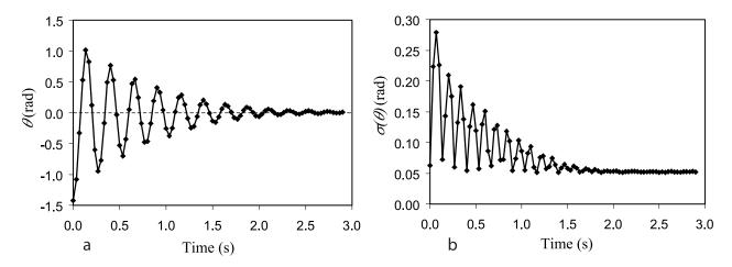
**Figure 3.** (left) Deflection angle  $\theta$  as a function of time during an oscillation measurement of the Telltale. (right) Standard deviation of the position of the Kapton part of the Telltale (blur), in the same measurement. This quantity should be proportional to the angular velocity of the Kapton part of the Telltale.
