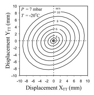
**Figure 6.** Displacement diagram for the Kapton part of the Telltale on Mars, under the conditions indicated. The negative  $Y_{TT}$  axis represents  $\beta = 0^{\circ}$  orientation.
