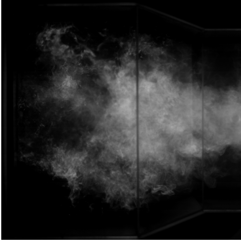
Figure A.5: Single frame from 1000 Hz high speed video of flame chemiluminescence at t= 51 ms.
