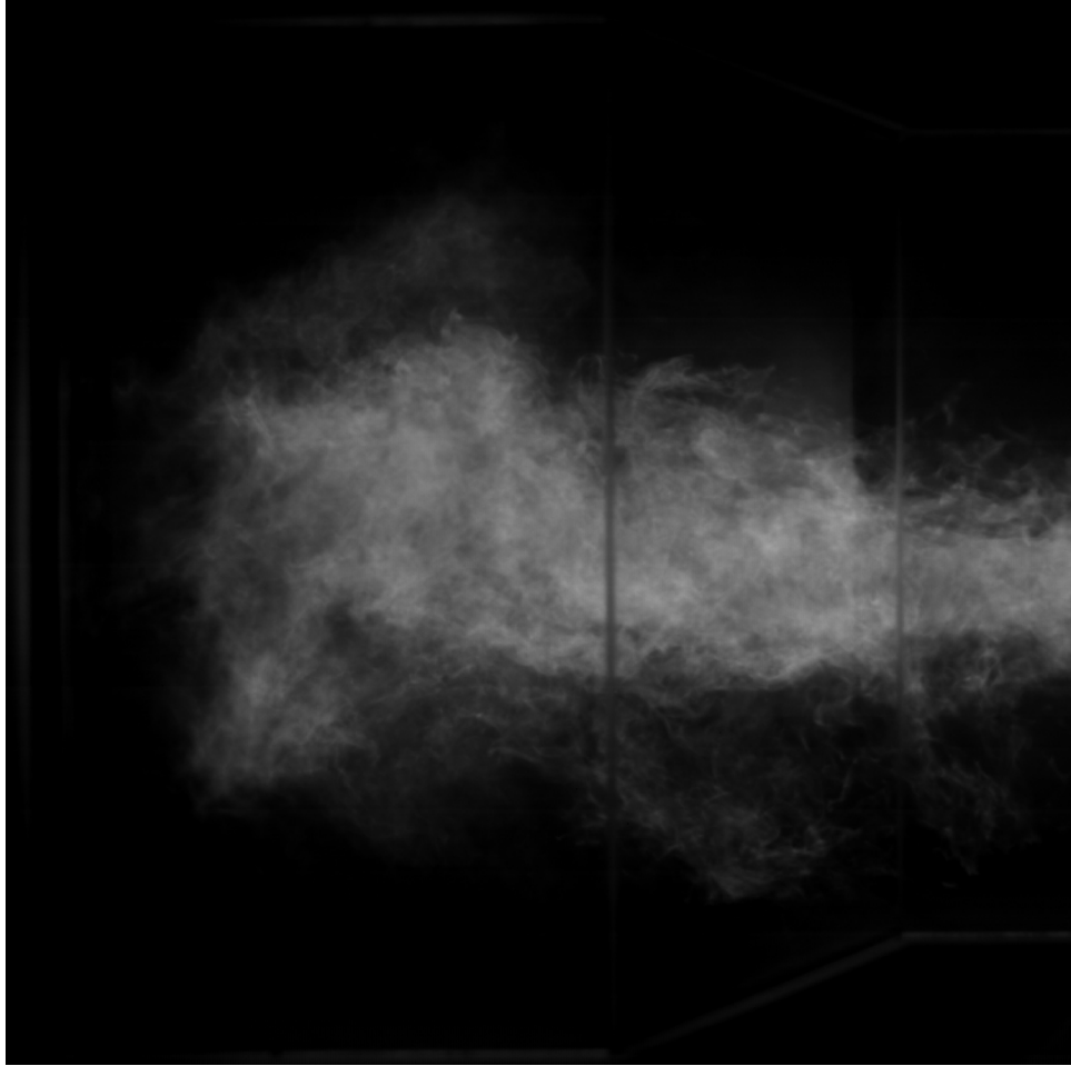
Figure A.1: Single frame from 1000 Hz high speed video of flame chemiluminescence at t = 47 ms. Run conditions listed in Table 4.4
