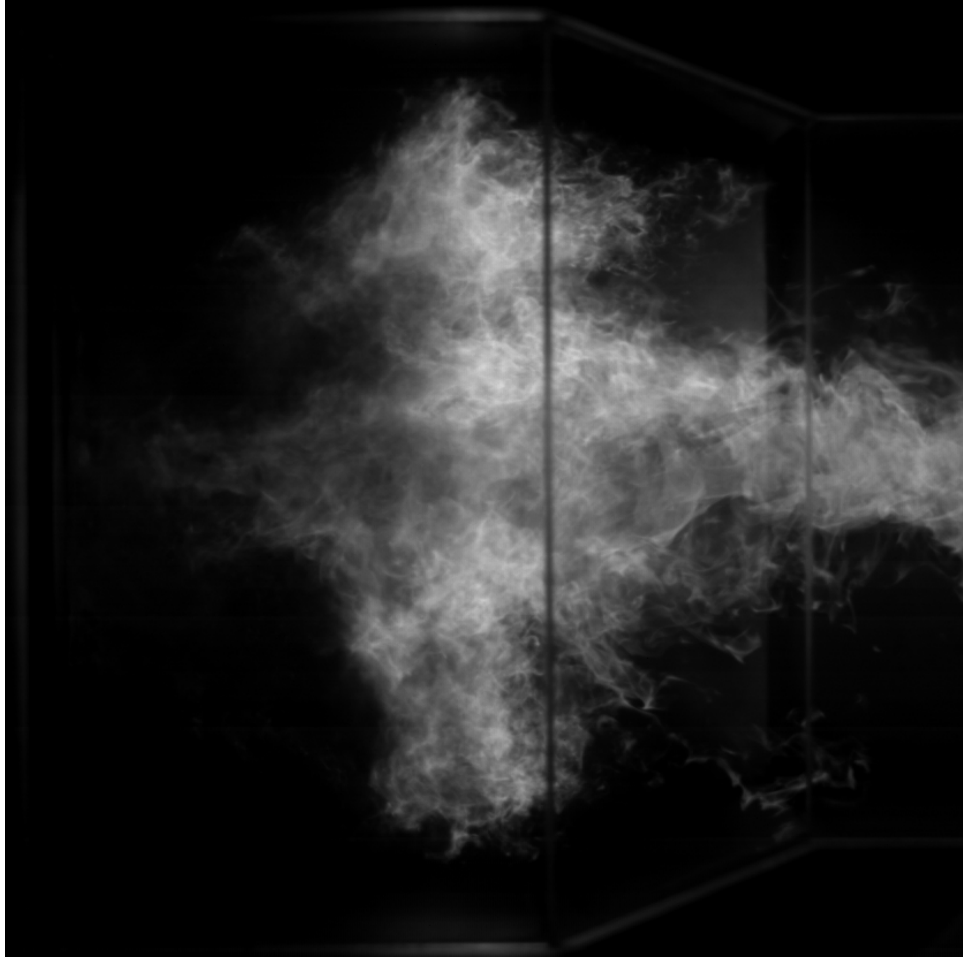
Figure A.9: Single frame from 1000 Hz high speed video of flame chemiluminescence at t= 55 ms.
