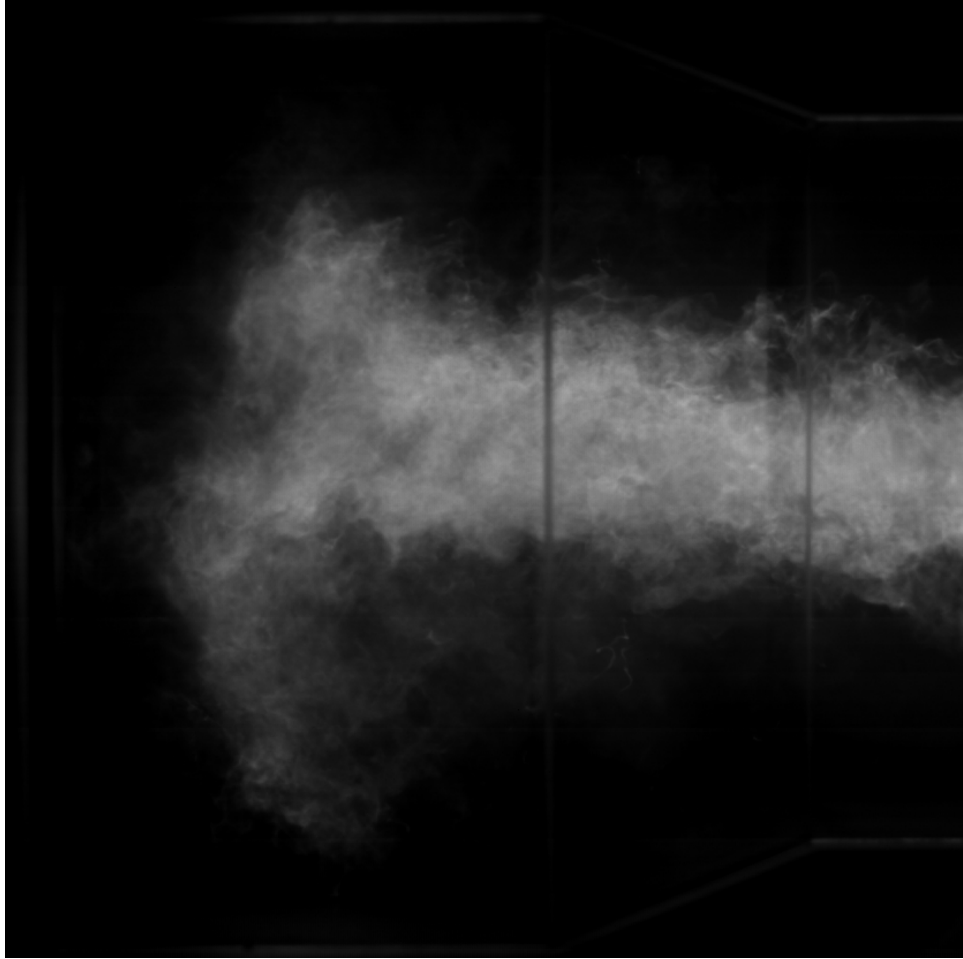
Figure A.2: Single frame from 1000 Hz high speed video of flame chemiluminescence at t= 48 ms.
