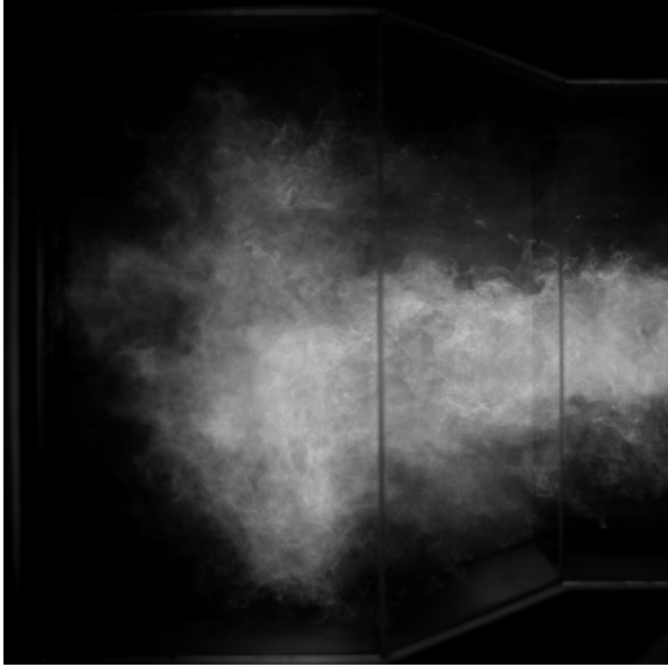
Figure A.15: Single frame from 1000 Hz high speed video of flame chemiluminescence at t= 61 ms.
