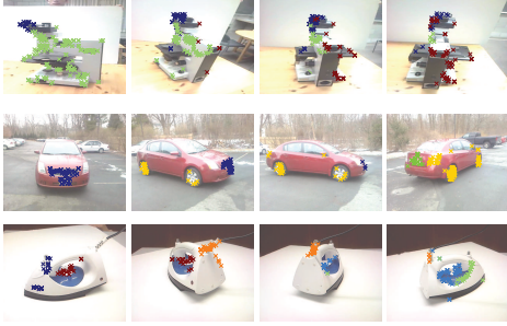
Figure 3.2: Examples of candidate parts of different object classes. Image patch features are denoted by “x”. x’s of the same color indicate that they belong to the same candidate part.
