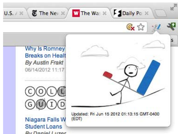
Figure V-5 Example Chrome extension with hindsight visualization. The icon in the browser provides persistent indication of the reader's history for the week, while clicking shows a larger view.
